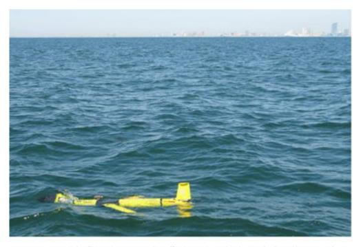
An autonomous glider floats about two miles off Atlantic City, after being deployed by a team from Rutgers University. Researchers are using the glider to sample ocean pH to help them understand how increasing carbon dioxide in the atmosphere is boosting levels of ocean acidity in the water.
